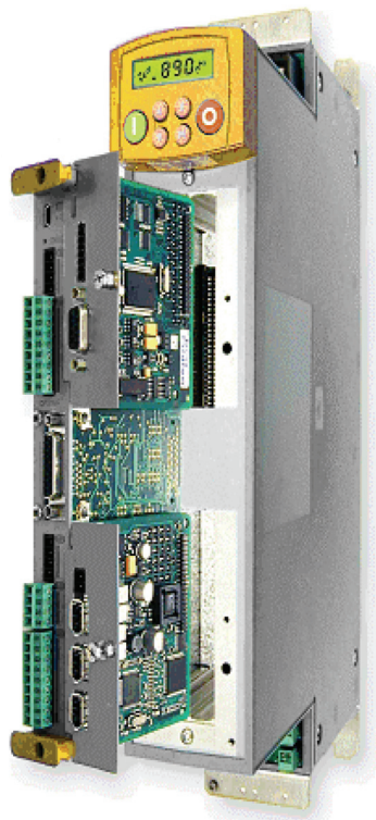
Figure 2. 890 showing Control Board withdrawn with Options fitted
